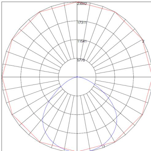
Maximum Candela = 23081.95 Located At Horizontal Angle = 60, Vertical Angle = 4
