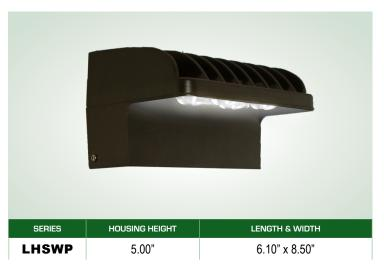
**MOUNTING** — Quick sheet metal mounting bracket connects to a standard J-Box. The bracket has a unique hanging feature to allow easy wire connections. After connections are made, the fixture swings up and is secured with with two retaining screws at the top of the fixture. An additional back box is available for applications requiring conduit entry (See Accessories).
